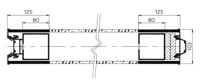
Horizontal Section Through Non-Stack Jamb and Telescopic Jamb
