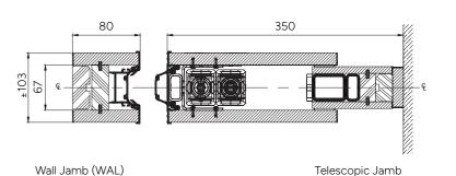
Horizontal Section Through Standard Panel (NE)
