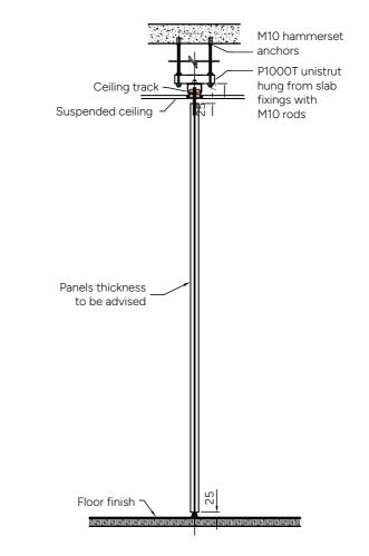
Vertical Section of **Panel & Track Fixing**
